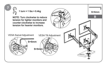
Tighten the bolt with the Allen Key to make the tilt and swivel adjustment.
